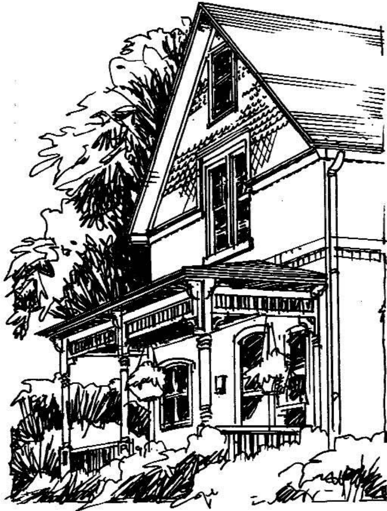
C-12 Upper floor space within roof structure
